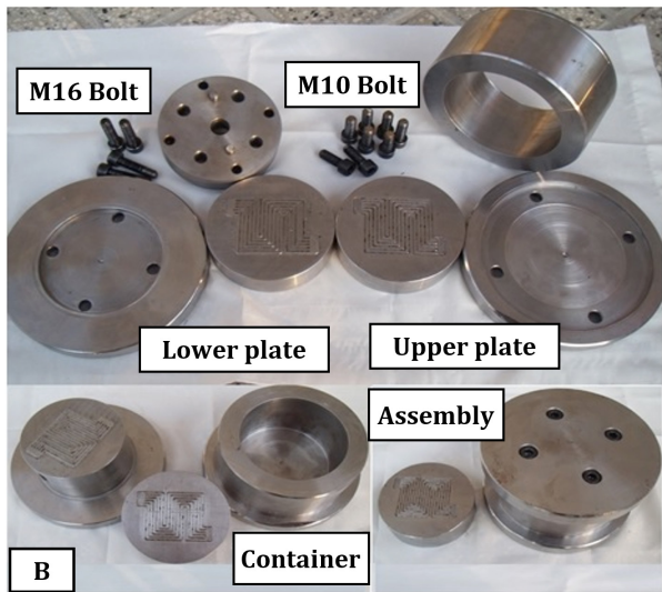
Fig. 7. Set of dies used to forming the plates, A) set template with 2 mm clearance between the punch and matrix, B) die with 0.01 mm clearance
