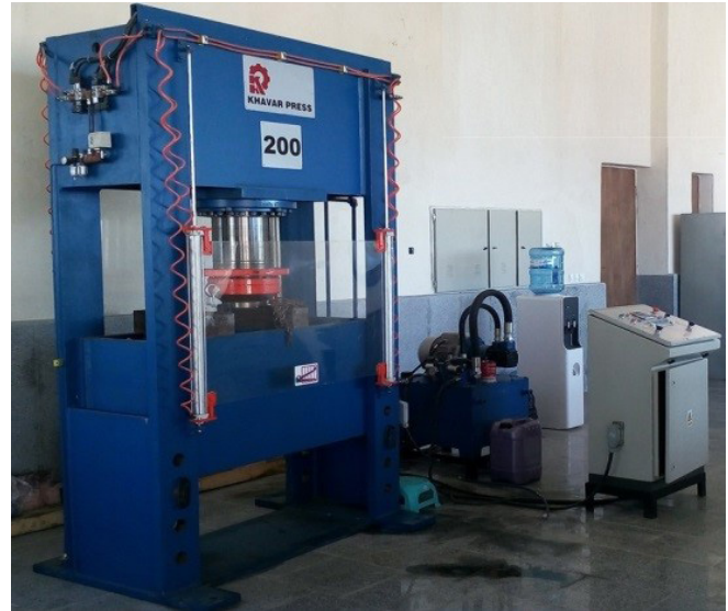
Fig. 6. Applied hydraulic stamping device for acting force on the die with capacity of 200 ton
