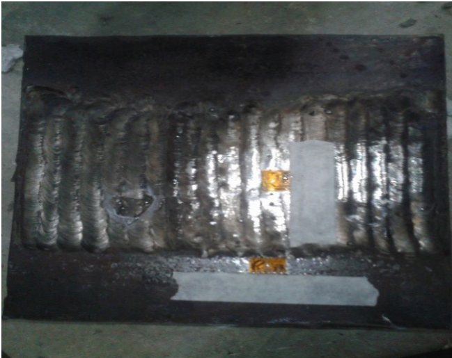
Fig. 14. How to apply strain gauges on the sample.
