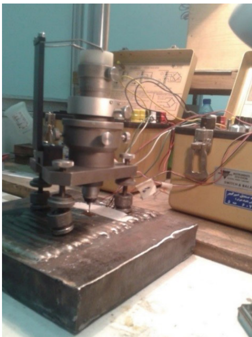
Fig. 16. How to test to measure residual stresses.
