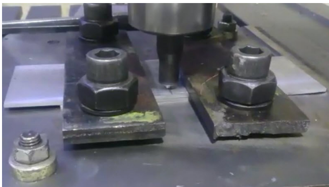
Fig. 3. Experimental demonstration of friction stir lap welding
