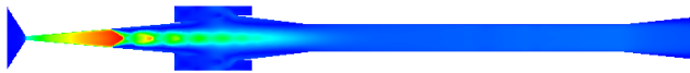
Fig. 30. Mach contour in designed wind tunnel for Mach number 6 in the pressure ratio of 35
