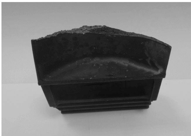
Fig. 3. The fractured blade
