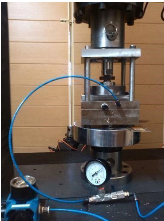
Fig. 9. Designed setup for leakage test.
