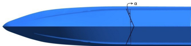
Fig. 13. Definition of the step forward angle
