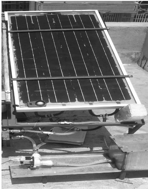
Fig. 2. Experimental setup picture of PV/T collector located in Department of Mechanical Engineering, University of Sistan and Baluchestan
