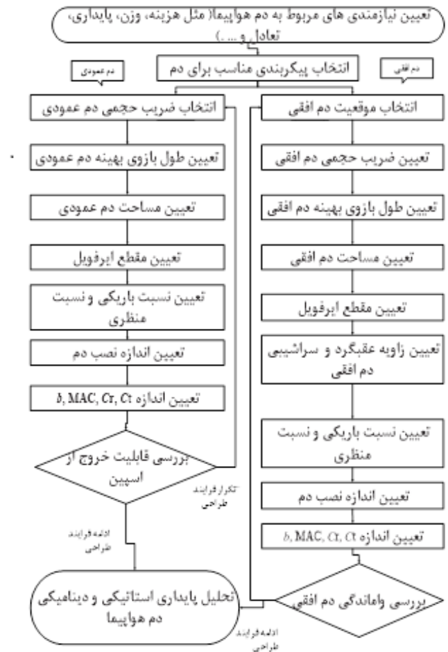
Fig. 3. Block diagram of tail design process
