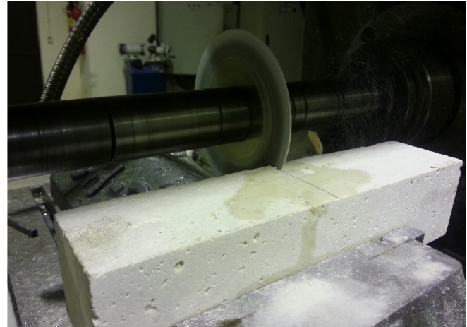
Fig. 3. Creation crack in SENB specimen
