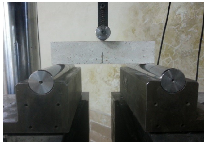
Fig. 4. The geometry and loading of the cubic specimens for SENB tests
