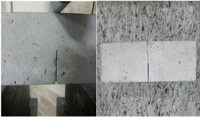
Fig. 5. Loading and crack growth in SENB specimen
