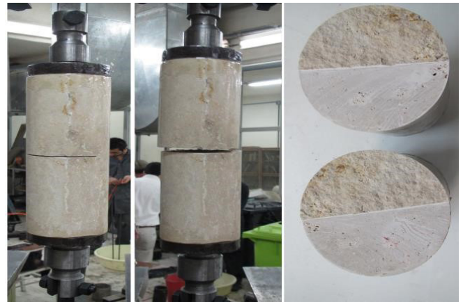
Fig. 6. Fracture and crack growth in DT specimen
