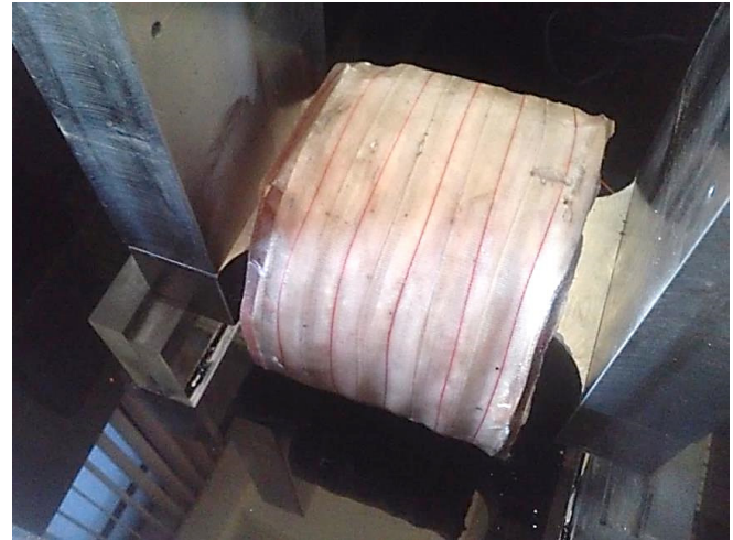
Fig. 9. Core and yokes with assembled winding
